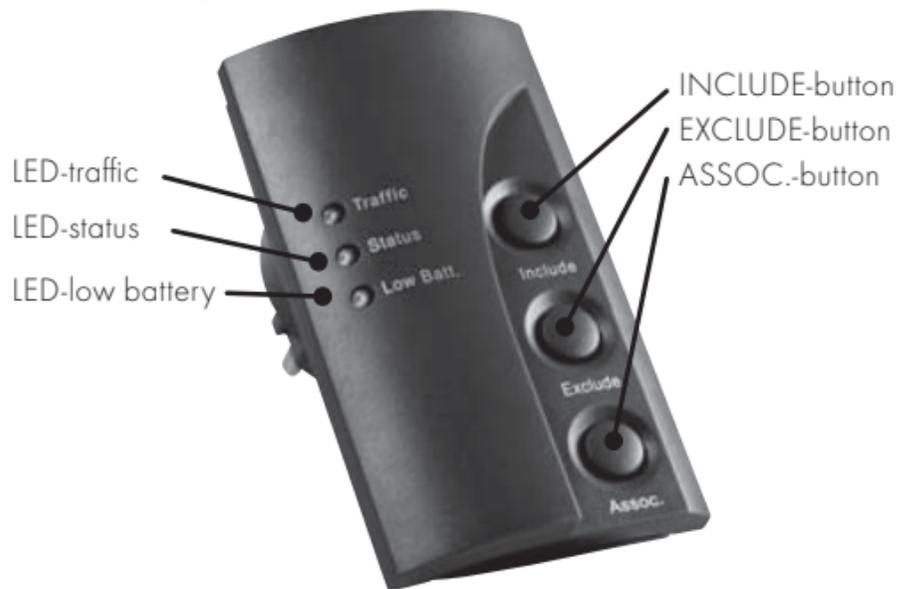
The **INTERACT<sup>3</sup>** wireless switching centre has the task of organizing the radio system or rather the network. Such a wireless switching centre finds application if you use more than one controller (wireless wall switch or remote control) in the network. The switching centre simplifies the handling, coordinates in the radio-network and monitors the battery level of the battery-operated devices and takes over a multitude of management functions in the network.
