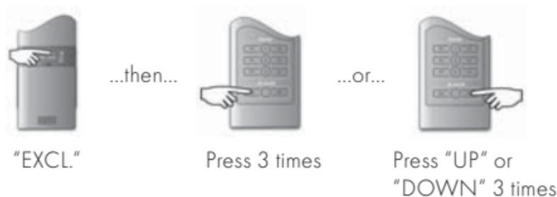
Press the **"EXCL."** button for five seconds (red/yellow/green blink), then press 3 times on the **"ALL ON"** button (prompt blinking) and 3 times on the **"ALL OFF"** button. (remote control) or 3x "UP" or 3x "DOWN" (wall switch).
