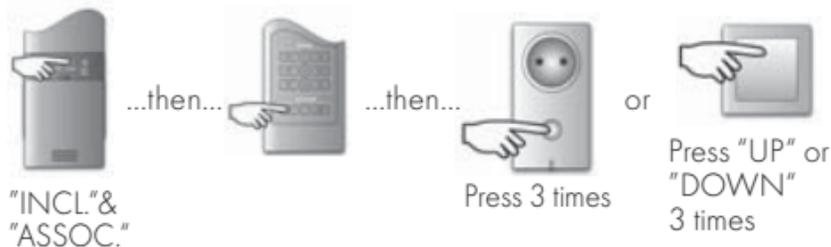
1. Press **"INCL." & "ASSOC."** buttons on the main remote control (blinks green)
