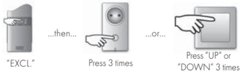
Press the **"EXCL."** button on the remote control for two seconds (blinks green) and then triple-press the **"UP"** or **"DOWN"** button or the **"FUNCTION"** button of the target equipment within 1.5 seconds.
