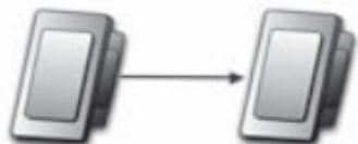
By dimming of the first actuator, for instance, by 10 %, all other actuators are likewise dimmed by 10 %. However, each actuator can still be manually adjusted.
