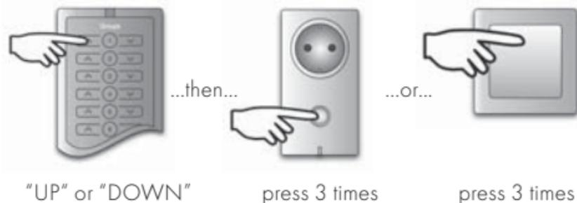
Press 3x on **“UP”** or **“DOWN”** on the desired group/ scene of the remote control or the wireless wall switch (blinks green) and then press 3x on the devices. The device is automatically associated with the selected group/ scene or the wireless wall switch.
