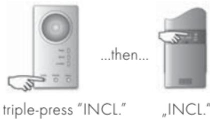
1. Triple-press the **"INCL."** button at the switching centre/server within 1.5 s.
