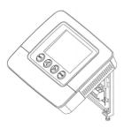
Tighten the 2 captive screws on the underside of the unit.
