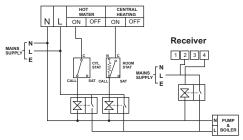
SSR303 receiver controlling a secondary heating zone on a fully pumped system with existing programmer and two spring return valves with auxiliary switches
