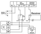
SSR303 receiver replacing a conventional room thermostat on a fully pumped system with an existing programmer and 3 port mid-position valve.
