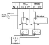
SSR303 receiver replacing a conventional room thermostat on a fully pumped system with existing programmer and two spring return valves with auxiliary switches
