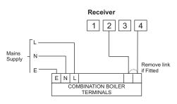
SSR303 receiver controlling typical combination boiler installation. For precise termination connection information please refer to the boiler manufactures instructions.
