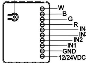
1. Connect the R.G.B.W. Color LED Dimmer according to wiring diagram.
