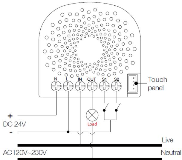
**Note:** The “IN” terminal should be connected to the “Live” of AC 120V/230V power wire.
