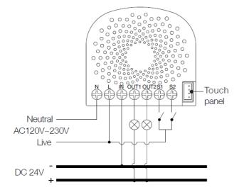
Note: The "IN" terminal should be connected to the "-" of DC 24V input.
