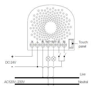
$\textbf{Note:} \ \ \text{The "IN" terminal should be connected to the "Live" of AC 120V/230V power wire.}$
