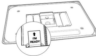
4. Mount the Swipe back into the back case by sliding the device up.
