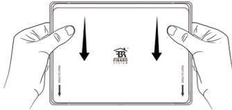
3. Remove paper strip protecting the batteries.
