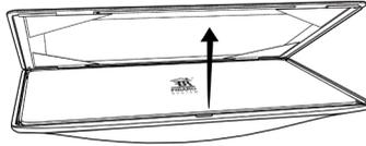
2. Unmount the Swipe from the back case by sliding the device down.
