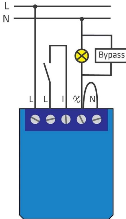
① NOTE: When installing the Mini Dimmer, with LED loads, in a 2-wired installation, if the load connected to the output starts flickering, we recommend you use a Bypass.
