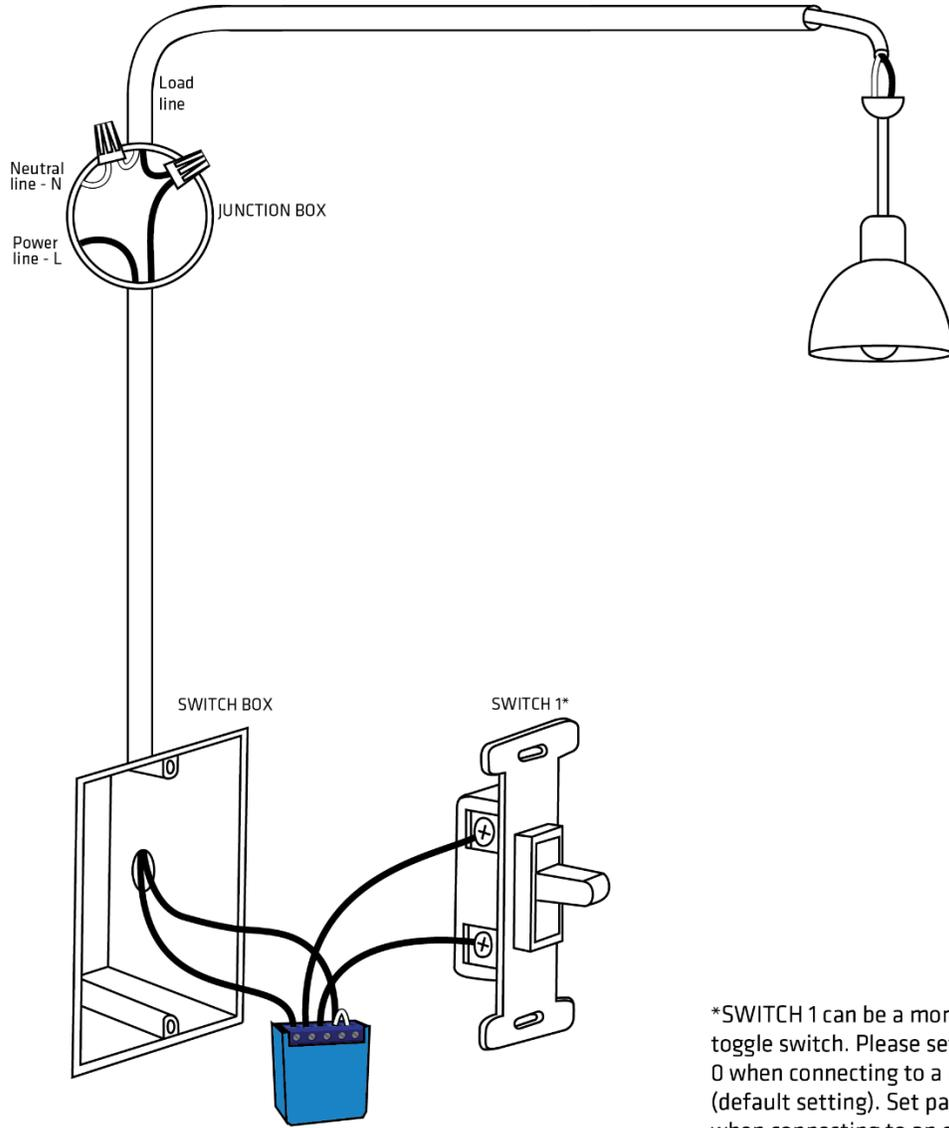
\*SWITCH 1 can be a momentary switch or a toggle switch. Please set parameter 1 to value 0 when connecting to a momentary switch (default setting). Set parameter 1 to value 1 when connecting to an on/off toggle switch. Please see the Configuration Parameters chapter for more information about advanced parameter settings
