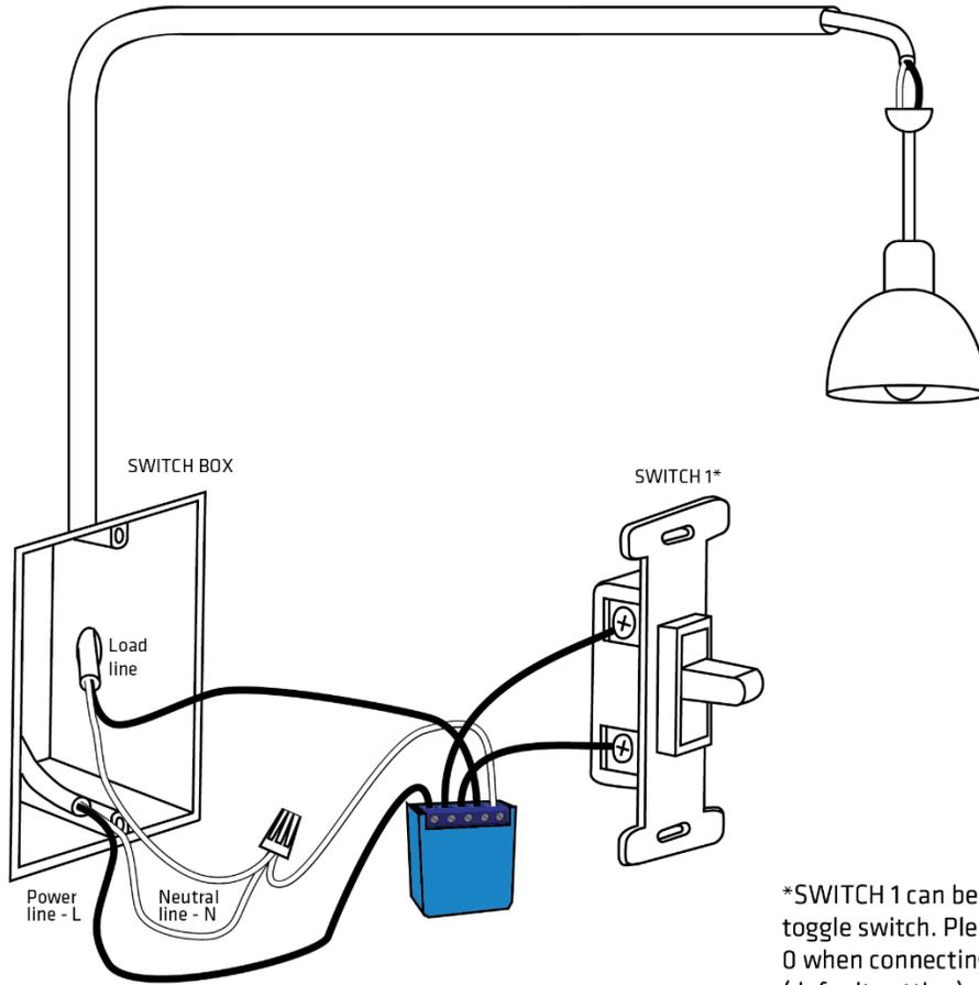
\*SWITCH 1 can be a momentary switch or a toggle switch. Please set parameter 1 to value 0 when connecting to a momentary switch (default setting). Set parameter 1 to value 1 when connecting to an on/off toggle switch. Please see the Configuration Parameters chapter for more information about advanced parameter settings
