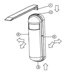
Replace the new battery and install the cover back.
