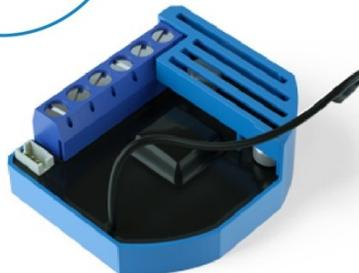
*The Qubino Flush Shutter DC device is ideal for remotely controlling 12–24V DC motors of blinds, rollers, shades, venetian blinds and similar sunscreens.*
