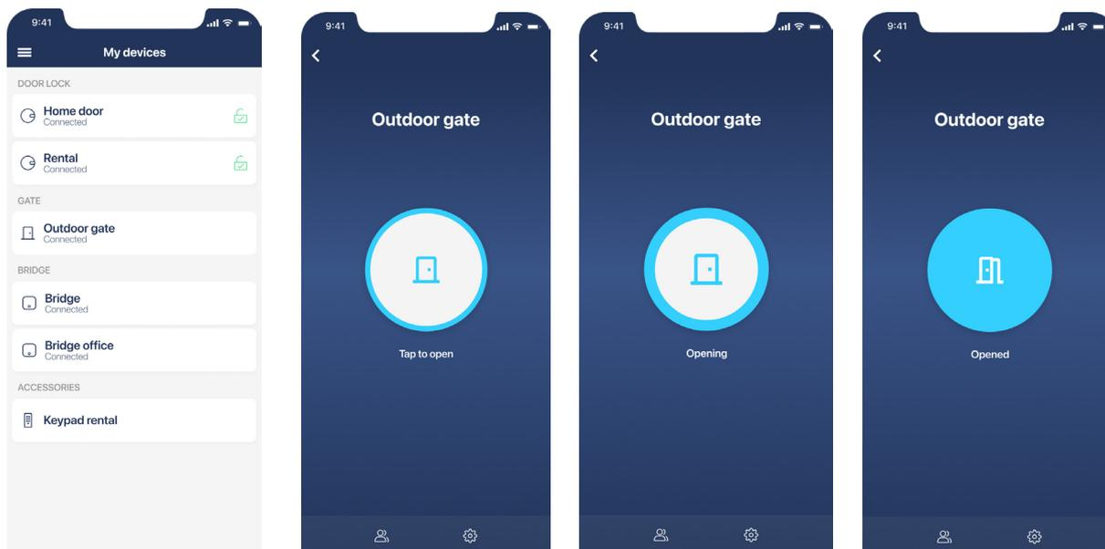
Tap the centre button to unlock the connected relay device.
