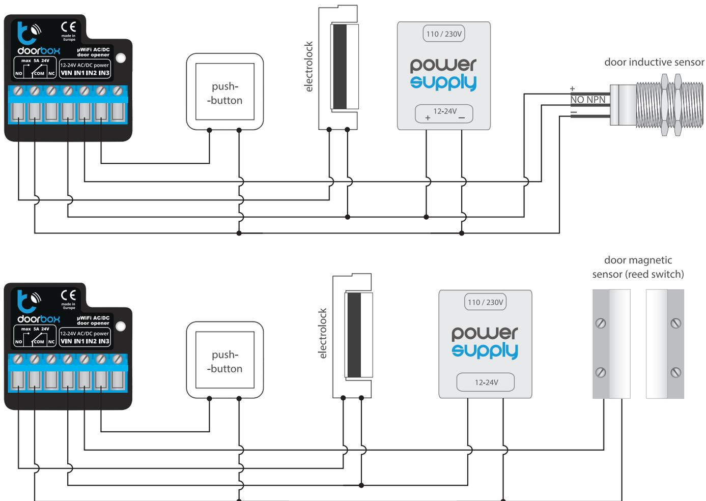
Start by connecting the +12V or +24V power wire (red or black with a white dotted line) to the VIN port and the ground (black) to the COM port.
